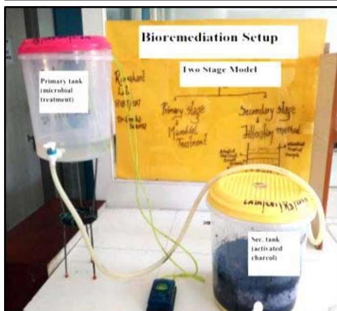
Figure 1. Experimental set-up for two stage model
